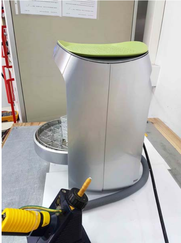
Picture #6 ESD immunity test setup
