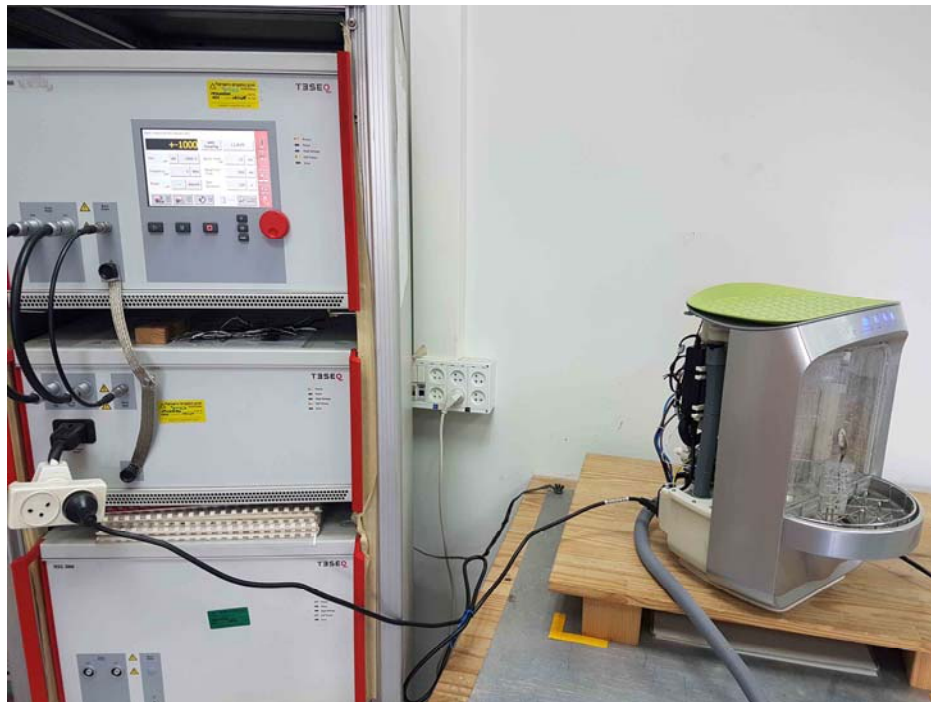
Picture #3 EFT, Surge & Voltage interruptions immunity test setup
