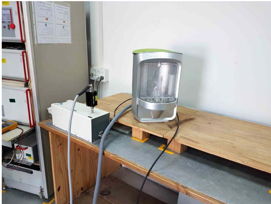
Picture #4 RF Conducted immunity test setup
