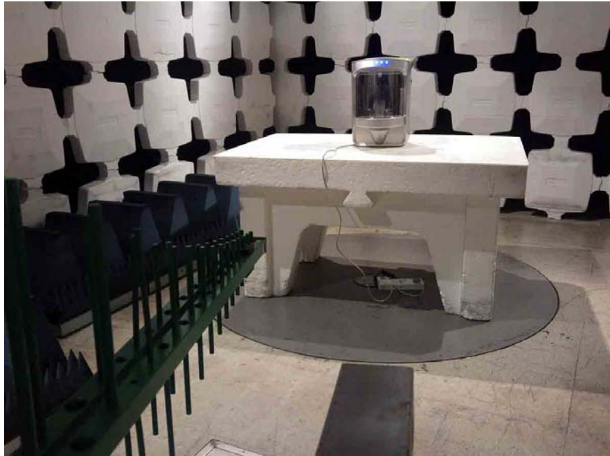
Picture #1 Radiated emission test setup
