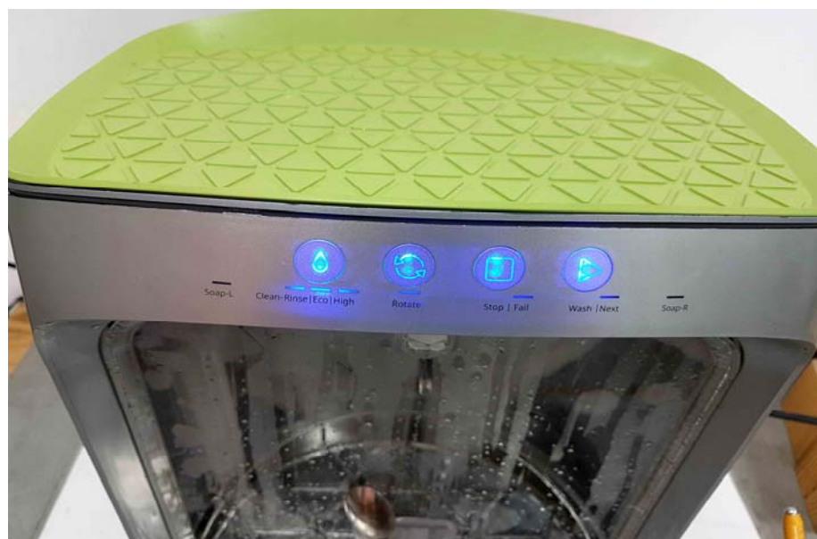
Picture #5 ESD immunity test setup. Tested point - control panel
