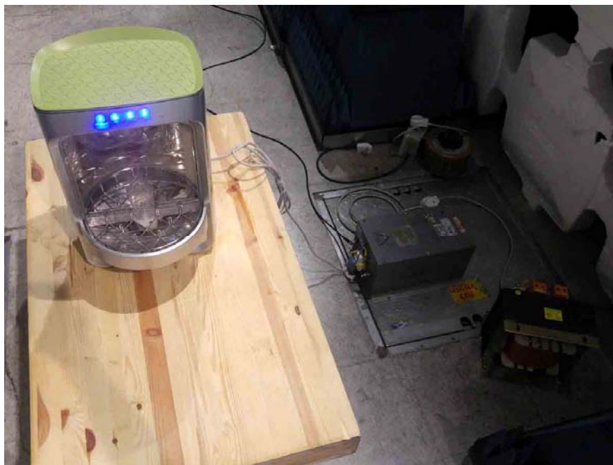
Picture #2 Conducted emission test setup per EN55014-1
