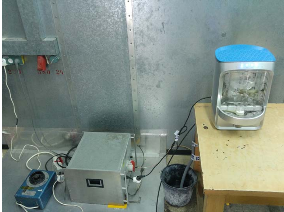
Picture #2 Conducted emission test setup per FCC Part 15
