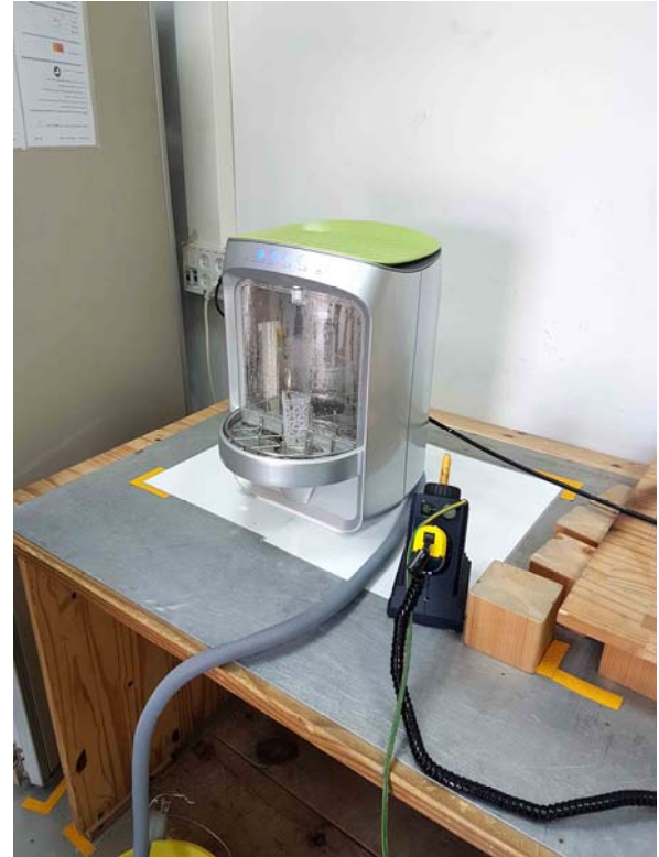
Picture #6 ESD immunity test setup
